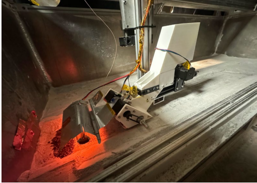
Figure 3: Road surface material deployment and curing prototype mechanism
