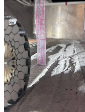
Figure 5: 10 psi tweel loading of the subsurface layered improvement resulting in a 1.5cm impression. Similar testing was conducted on compacted and uncompacted MTU-LHT-1A. The resulting wheel sinkage was measured to be 2 cm and 3.4 cm respectively.
